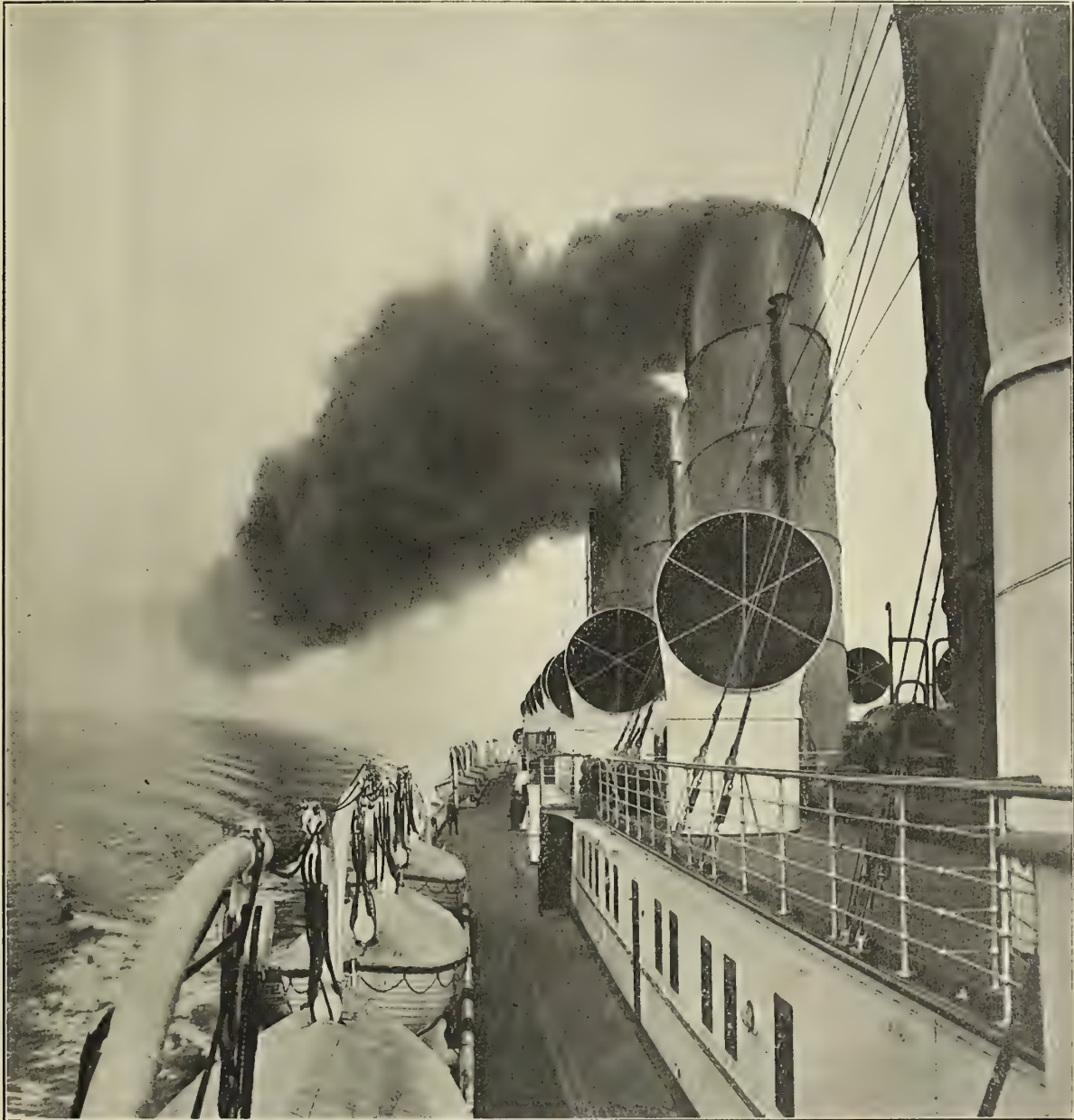
THE MAURETANIA AT FULL SPEED AT SEA, SHOWING THE ARRANGEMENT OF VENTILATORS AND FUNNELS.
